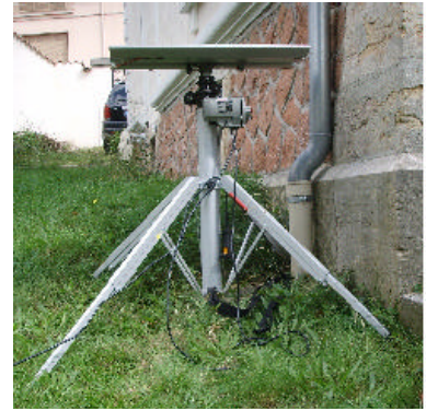
4 adjustable legs to use in uneven terrain, stairways etc...
